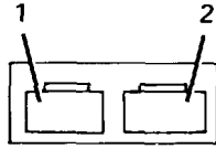
Wiring Face PROGRAM SWITCH (C1)
